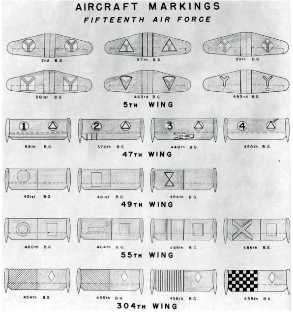
The sketch above shows the markings on the horizontal stabilizers (upper B-17, lower B-24) with their corresponding Bombardment Group markings; the sketch on the following page shows the vertical tail markings. (HF)
