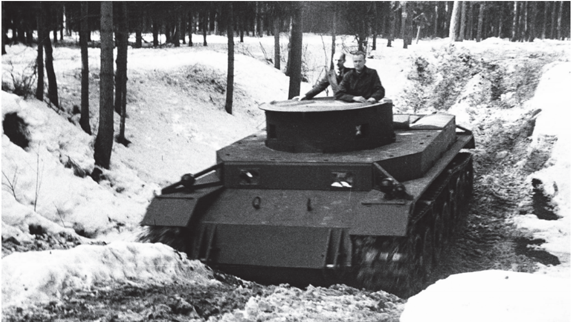
One of the two VK 3001 (P) testing on the running-in track in winter 1941/42. The vehicles were not fitted with turrets. Instead, an equivalent weight was mounted for chassis testing. [Archive ECS]
