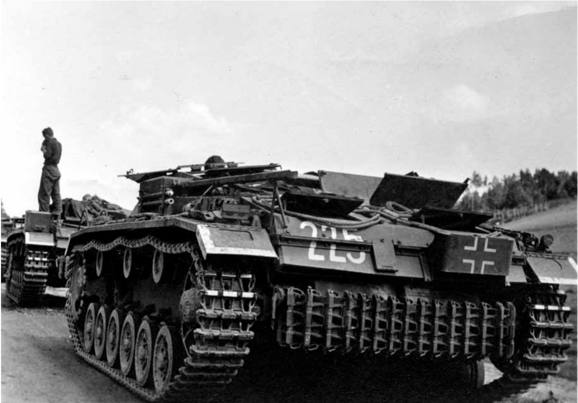
StuG III Ausf D / Armored smoke candle discharger on the stern and the distance light on the left track guard can be seen clearly / Note the new antenna mount and the visibility marking on the mud flaps / Engine and ventilator maintenance hatches are open / Alkett, 5. - 10.1941
