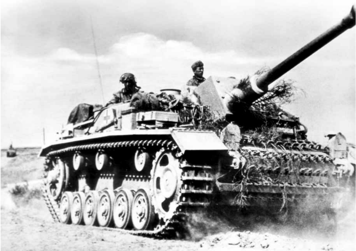
StuG III Ausf F (L/48) / Troops believed that additional spare tracks on the bow would reinforce the armor / Alkett, 6.1942
