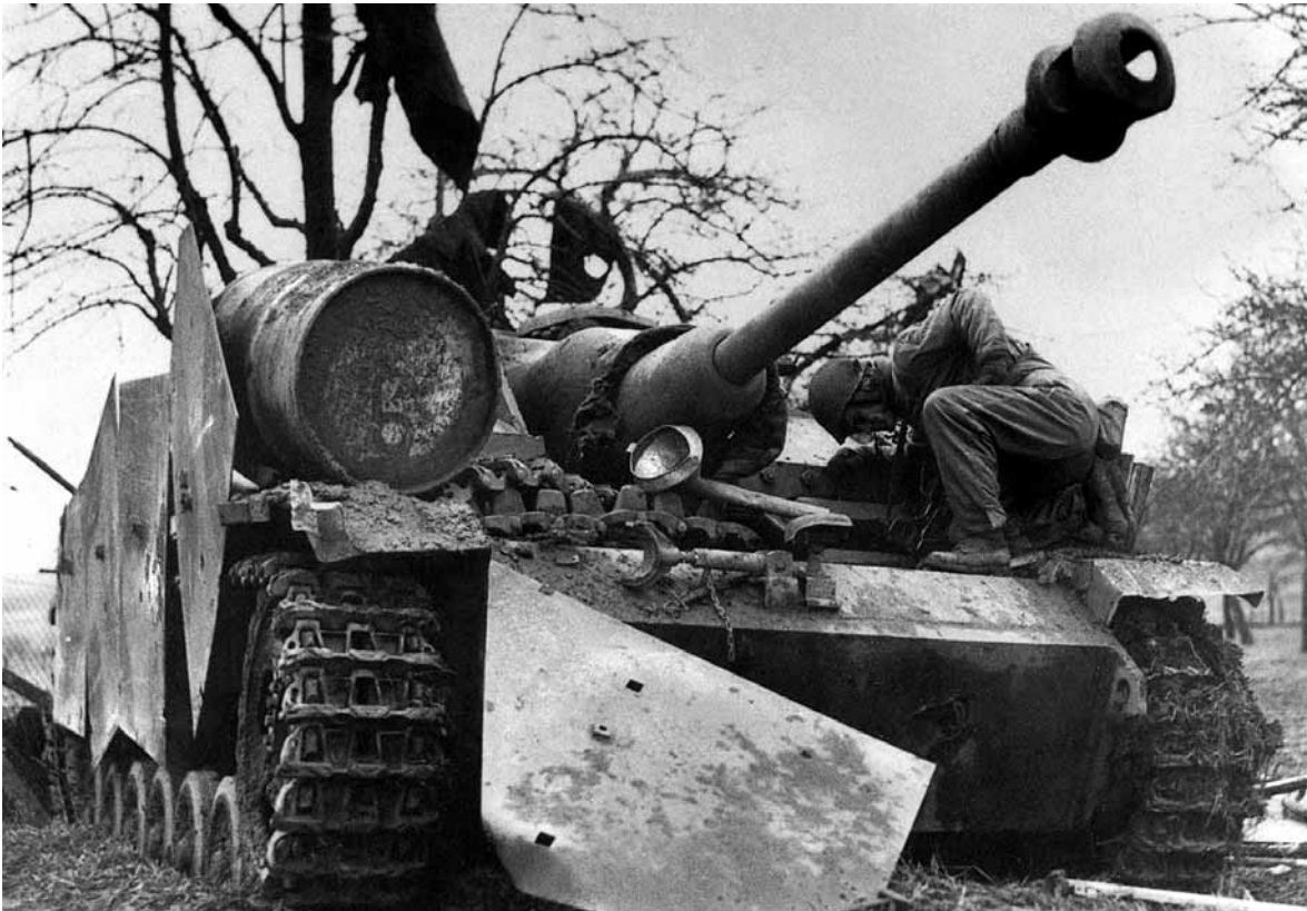
StuG III Ausf G / An American trooper inspecting the vehicle following the Ardennes Offensive / Attachments for armor skirts modified in the field and travel clamp retrofitted / Alkett, 9. - 10.1944
