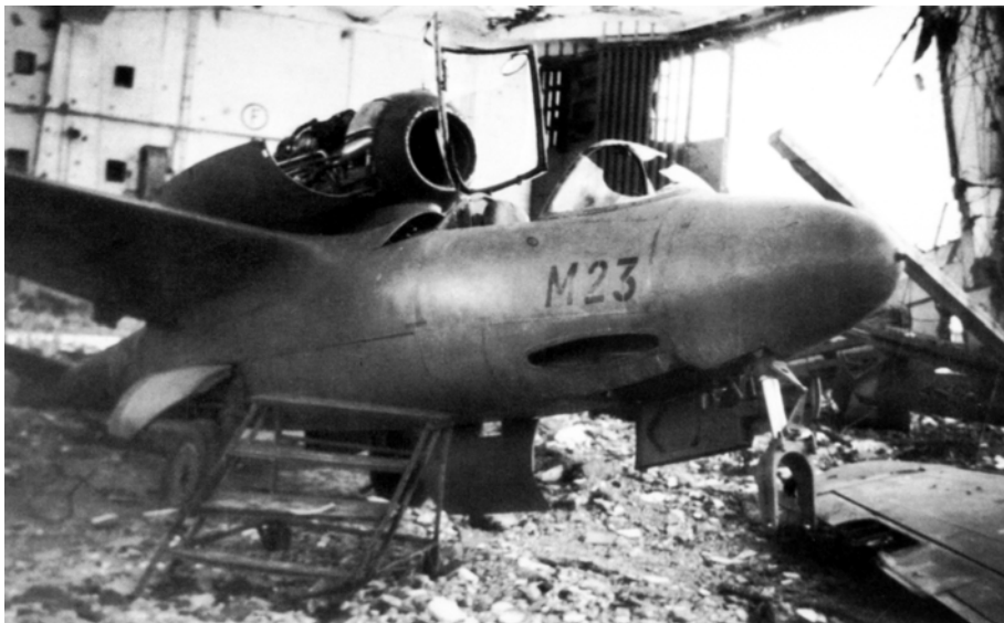
WNr 220006 (M-23) was captured on 1 st May 1945 at Munich-Riem. Without its armament and nose wheel, the machine tilted to the rear.
